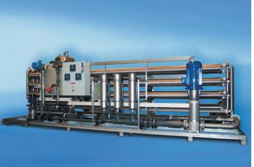
Reverse Osmosis Systems Dulcosmose® Series BW are specifically designed for brackish water desalination for drinking water supply as well as for industrial applications. Using state of the art low-pressure membranes, a system salt rejection rate of up to 99 % and a recovery of up to 80 % can be achieved.
